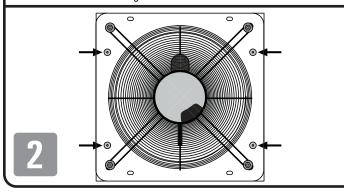
Using appropriate hardware (not provided) for your structure and the weight of your exhaust fan, secure the fan to your structure using the (8) pre-drilled holes on the flange. Exhaust fan must be mounted with the motor inside of structure, protected from the weather, and with capacitor on top as shown.
