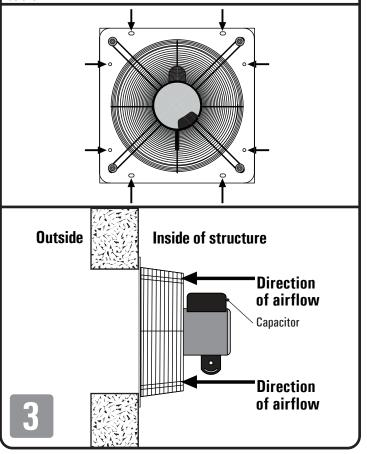
Using appropriate hardware (not provided) for your structure and the weight of the shutter, secure the shutter to the outside of your structure using the (8) pre-drilled holes on the flange. Louvers should open to the outside.
