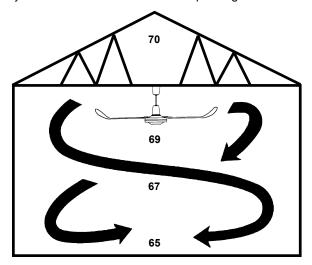
**THE AGRIFAN SOLUTION** - In winter AGRIFANS mix stratified air, forcing warmer air down to floor level, also reducing condensation. In summer vertical, turbulent air movement cools poultry and livestock. In all seasons, continuous vertical air circulation speeds drying of floors, bedding, walls and ceilings.
