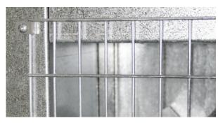
No cone models come with 1" x 2" wire mesh guards that are hot dip galvanized after welding. The guard is attached to the housing with poly guard clips to reduce noise and vibration.
