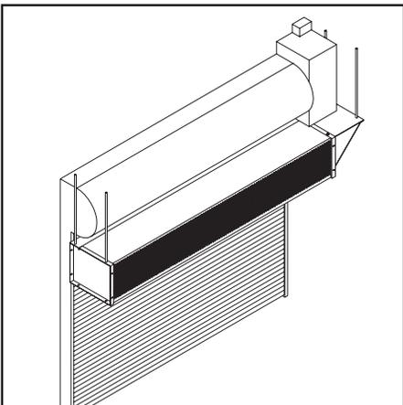
CEILING MOUNT with EXTENSION BRACKET for OPERATOR CLEARANCE
