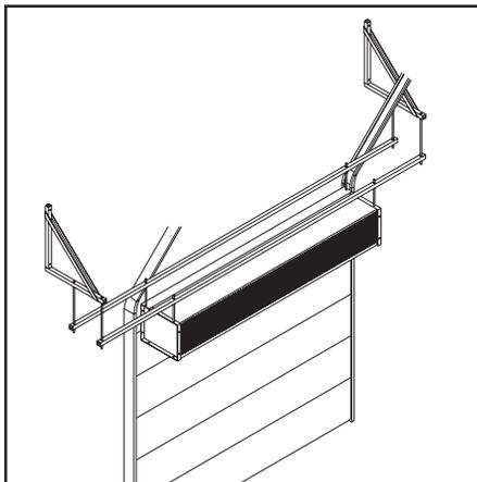
WALL MOUNT BRACKETS with THREADED ROD and STRUT for DOOR TRACK CLEARANCE
