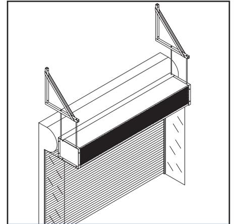
WALL MOUNT BRACKETS with CLEAR PVC SIDE SHIELDS
