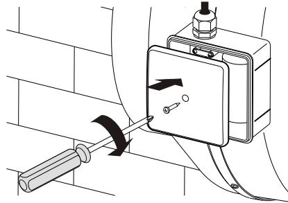
**Connection of the fan with box on cable**
