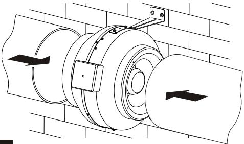
Installation of the fan with box on cable
