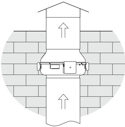
Installation of the fan with built-in box
