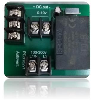
The JDAV010M is a 100-240v powered manual speed control for 0-10v speed control circuits.
